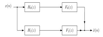
(a) Let the analysis filters be  $H_0(z) = 1 + 3z^{-1} + \frac{1}{3}z^{-2} + z^{-3}$  and  $H_1(z) = H_0(-z)$ . Find causal stable IIR filters  $F_0(z)$  and  $F_1(z)$  such that  $\hat{x}(n)$  agrees with x(n) except for a possible delay and (non zero) scale factor.(5 points)
