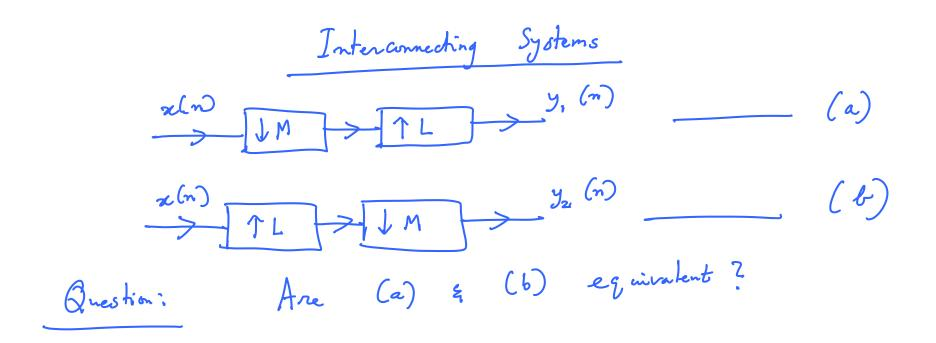
The systems (a) & (b) are equivalent if L and Theorem: M are relatively prime. i.e., gcd (L, M) = 1  $Y_{1}(z) = \frac{1}{M} \sum_{k=x}^{M-1} X(z^{k})$ Shetch  $Y_2(z) = \frac{1}{N} \sum_{m=1}^{M-1} X(z^{L/m} \omega_m^{kL})$ Claim: The set of numbers  $S_1 = \begin{cases} w_{M} \\ w_{N} \end{cases}$  distinct  $M^{th}$  roots of  $w_{N}$ . W.)  $S_2 = \begin{cases} w_{M} \\ y_{N} \end{cases}$   $0 \leq k \leq M-1$  is equal iff gcd(L, M) = 1
