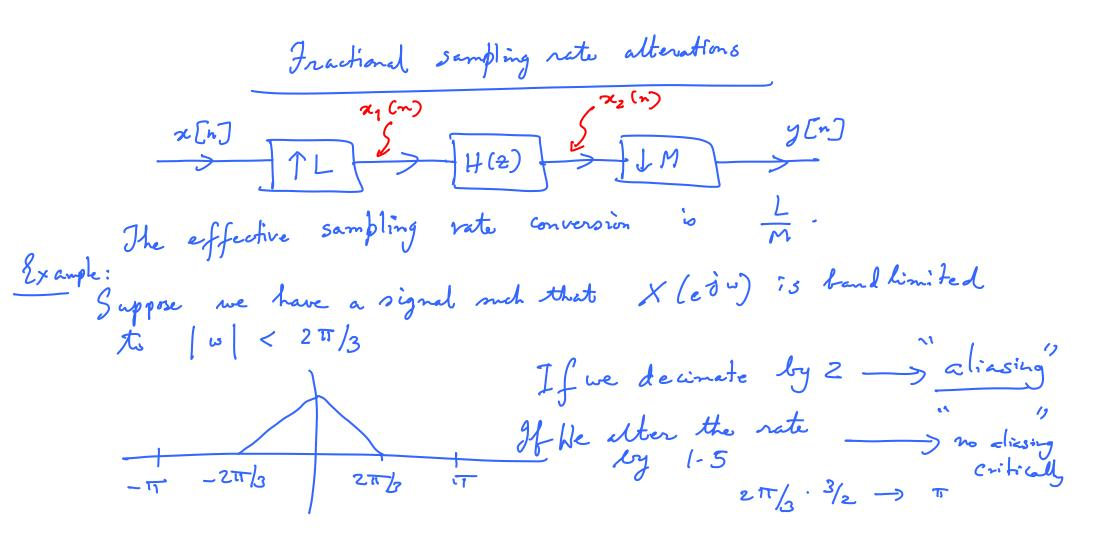
In general, we can reduce the Sampling rate by any national no Quality of the fitter H(3) determines the quality of the o/p. Stretched veroions of
