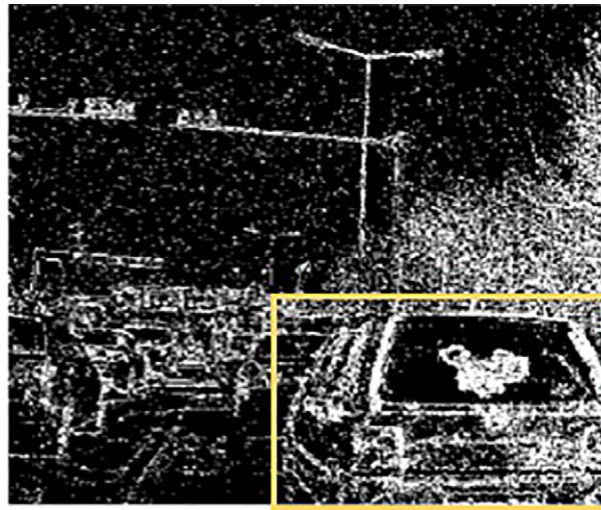
FIGURE 13 Object tracking for a moving camera. The image (available in the internet) is captured from DVS camera. As the camera was also moving, background generates a lot of clutters. Hence, tracking becomes a nontrivial task
